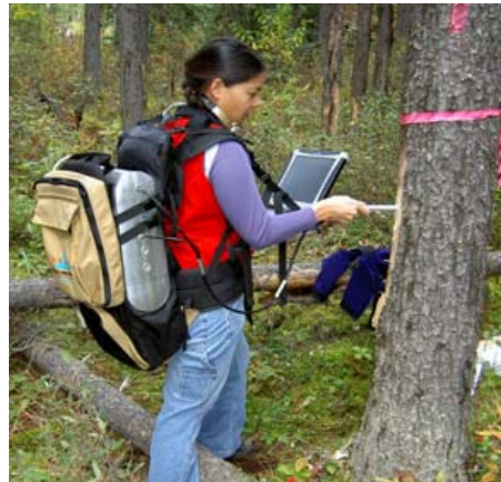
Collecting Vis-NIR spectrum in-field.
